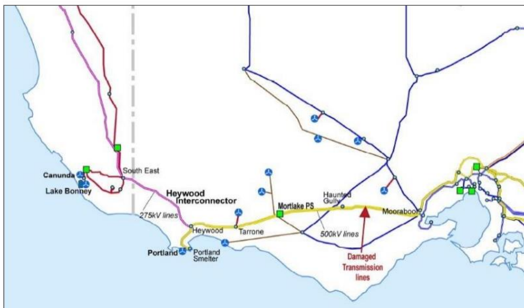
Figure 5: Map of impacts of 2020 Cressy towers failure. 5
