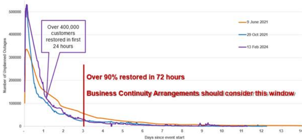
Figure 7: Chart of restoration during major power outages in 2021 and 2024. 9
